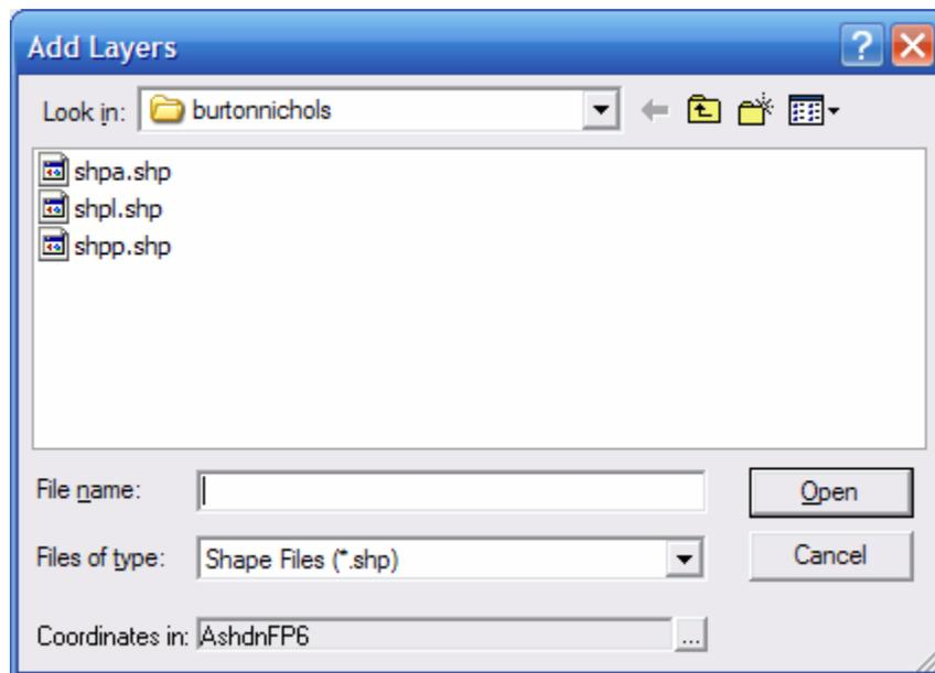
Note that our new coordinate system ‘AshdnFP6’ is listed as ‘Coordinates in:’. Change the “Files of type” drop down to (\*.dxf), then highlight the DXF you wish to import:
