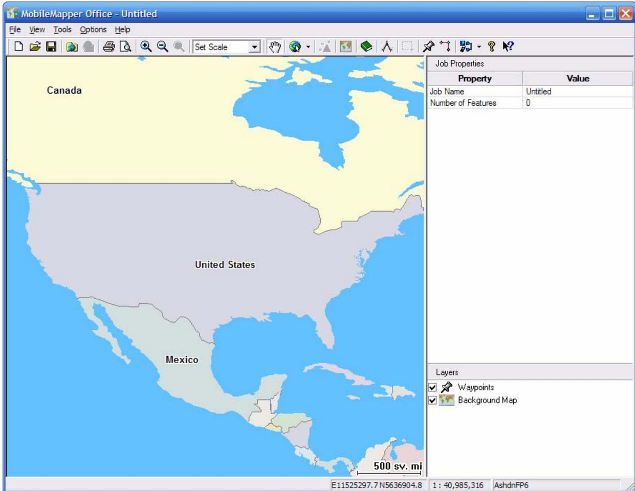
Now we can test our new local coordinate system by importing a DXF that uses the defined coordinate system. Select "File: Import" and browse for the DXF file (in this case it is named MarkDXFOut.dxf):
