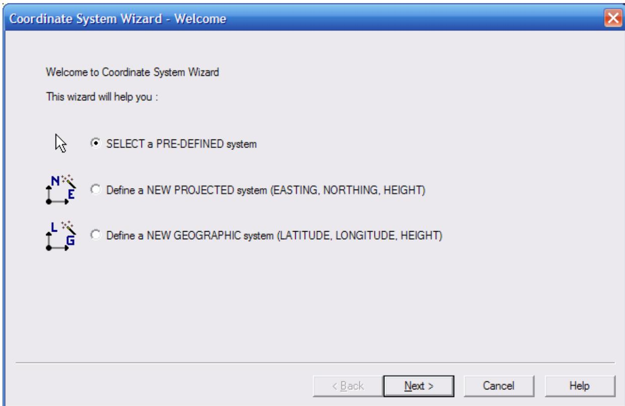
With “Select a Pre-Defined system” selected Press “Next”. Select “USA” and then pick the state plane coordinate system that makes sense for the job you are working with. In this case we computed offsets from Utah South NAD83 so you need to pick “NAD83” in the left box and “USA/NAD83/Utah (South)” in the right-hand box:
