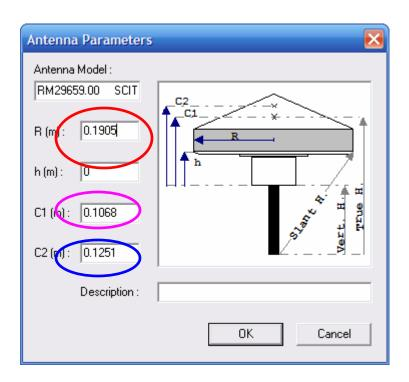
The h(m) value is ALWAYS "0" for NGS calibrations. (Don't ask why just do it!) C1 is the L1 offset, C2 is the L2 offset. Note that the radius is usually given in CM, whilst the C1 and C2 are always given in millimeters. GNSS Solutions ALWAYS expects the values in Meters.
