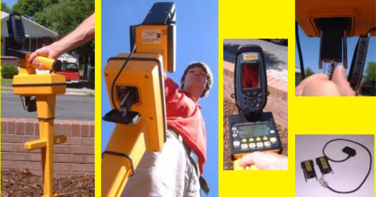
Adding a Thales Mobile Mapper™ GPS receiver to a 3M Dynatel™ locator automates the collection of marker position and attribute data. The Mobile Mapper Office software tool directly exports .DXF or .SHP files to industry standard cad and GIS applications.
