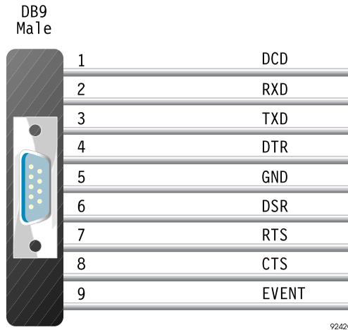
**Figure 1.4:** Port B Pin Assignments
