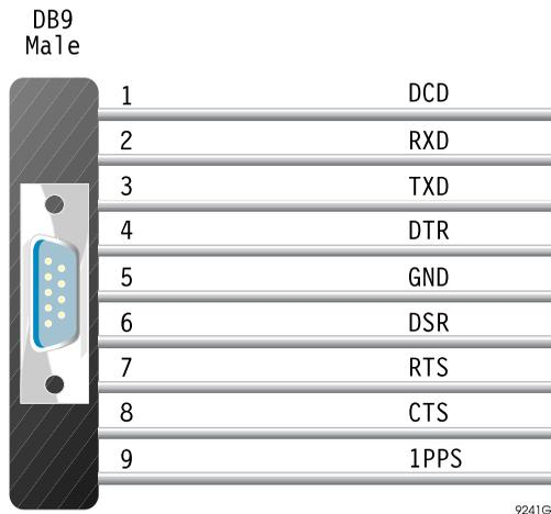
**Figure 1.3:** Port A Pin Assignments
