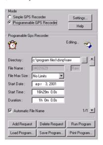
Directory: This text box is used to specify the directory to which you wish to record the data from the receiver. Clicking the button to the right opens a dialog box that allows you to navigate through the directory tree on your hard disk or a floppy disk, and select the desired destination directory.
