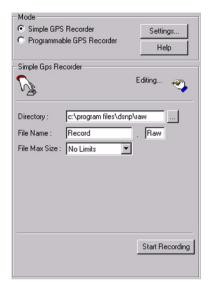
File Name: This text box is used to specify the name of the file to which you wish to record the data from the receiver.
