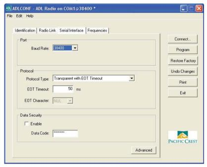
In this tab, you can configure the serial interface between the radio and external devices such as a computer running the ADLCONF software, a GPS receiver, or monitoring equipment.
