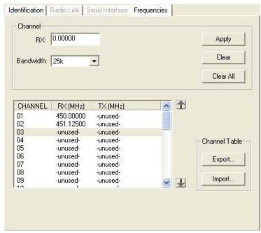
In the tab you can configure the radio for receive-only channels. When you first select the Frequencies tab, the current channel table shows the Rx frequency of Channel 01 in the RX field.
