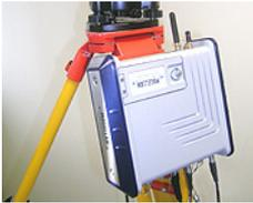
In land surveying applications, when used as a roaming base mounted on a tripod, the ProFlex 800 can be secured on one of the legs of the tripod using the lug located on its bottom side.
