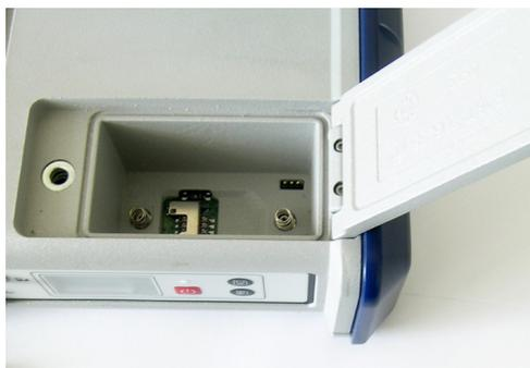
The battery used is a 7.4-V DC - 4600 mAh rechargeable battery. It is a standard model used in many camcorders. The battery is housed in a battery compartment accessible from above the ProFlex 800. The compartment door can be opened by lifting and then turning the quarter-turn finger screw counter-clockwise. The battery will automatically operate as a backup power source for the receiver if for some reason the external DC source used is removed from the DC power input.
