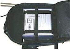
The ProFlex 800 is secured in a backpack when used as a rover for land surveying applications.
