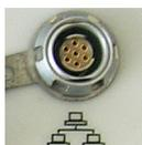
A Fischer, seven-contact female connector [7] allowing you to connect the ProFlex 800 to a local network (LAN). Through this connector, you may remotely control and monitor the ProFlex 800 from any computer connected to the Internet. Data may also flow through this port, in the same way as through a serial port.
