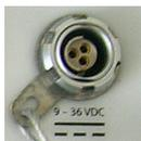
A Fischer, three-contact, female connector **[1]** allowing the ProFlex 800 to be powered from either the provided AC adapter (connect the cable extension between ProFlex 800 and the end of the AC adapter output cable), or an external 9- to 36-V DC power source through cable P/N 730477 (cf. base setup using an external radio transmitter).
