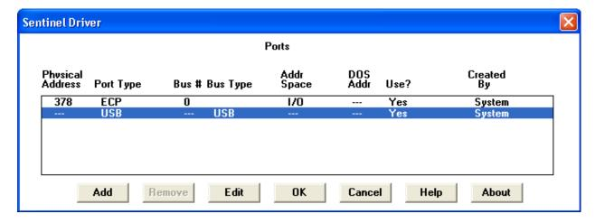
5. The following dialog will be displayed. Enter the I/O address of the PCI parallel port adapter into the "Bus Address" field.
