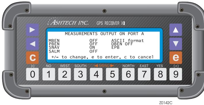
**Figure A.3.** Measurements Output on Port A Screen
