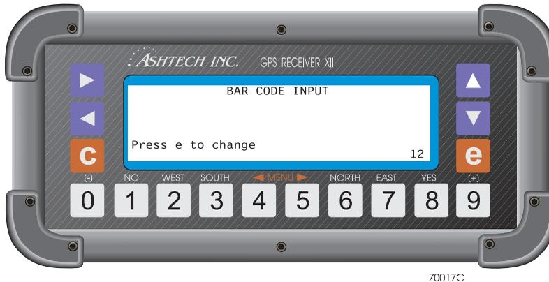
Figure 3.46. Screen 12 - Bar Code Control
