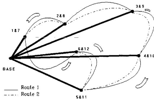
**Figure 5.4.** Pseudo-Kinematic, One Base, One Rover
