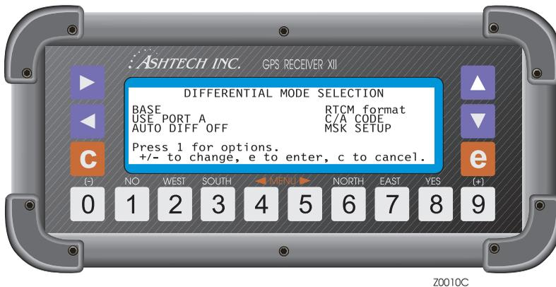
**Figure 5.7.** Differential Mode Selection Screen
