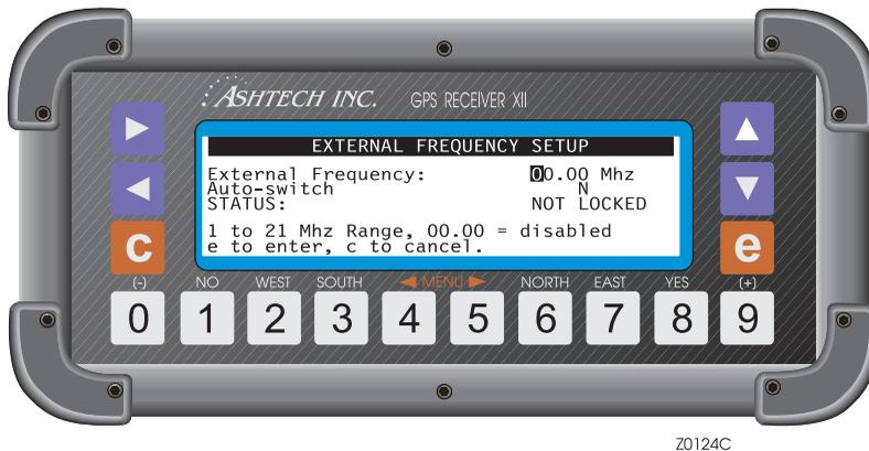
**Figure 3.13.** External Frequency Setup Screen
