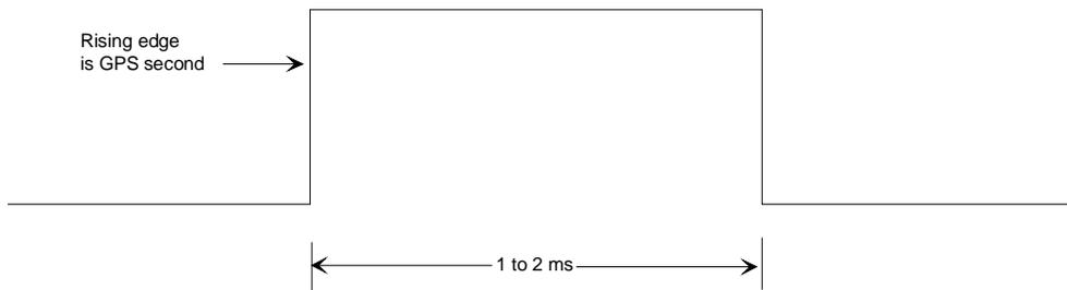
**Figure 3.14.** One PPS Signal Characteristics
