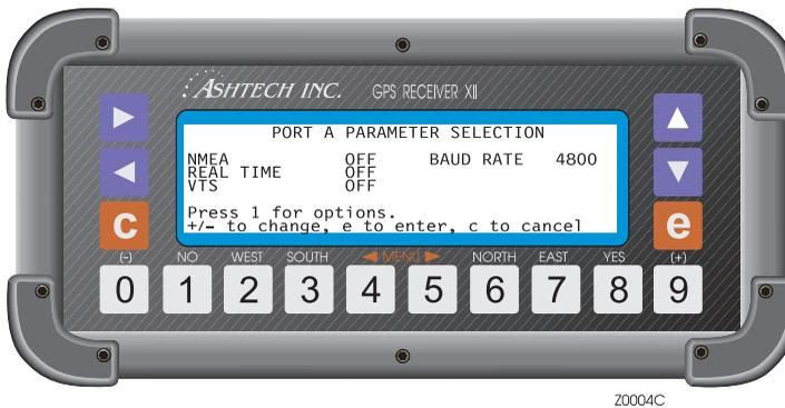
Figure A.5. Port A Parameter Selection Screen
