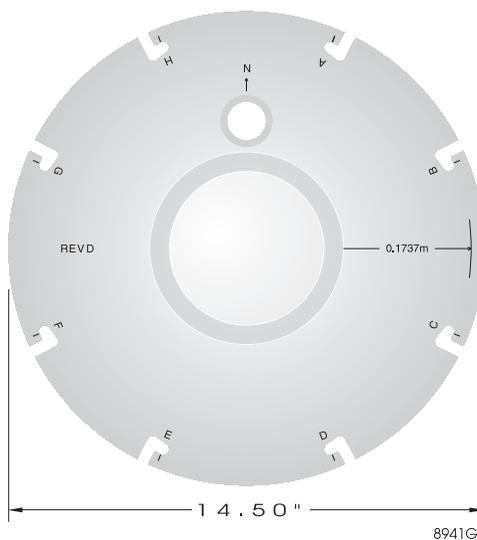
**Figure 1.4. Precision Antenna Platform, Top View**
