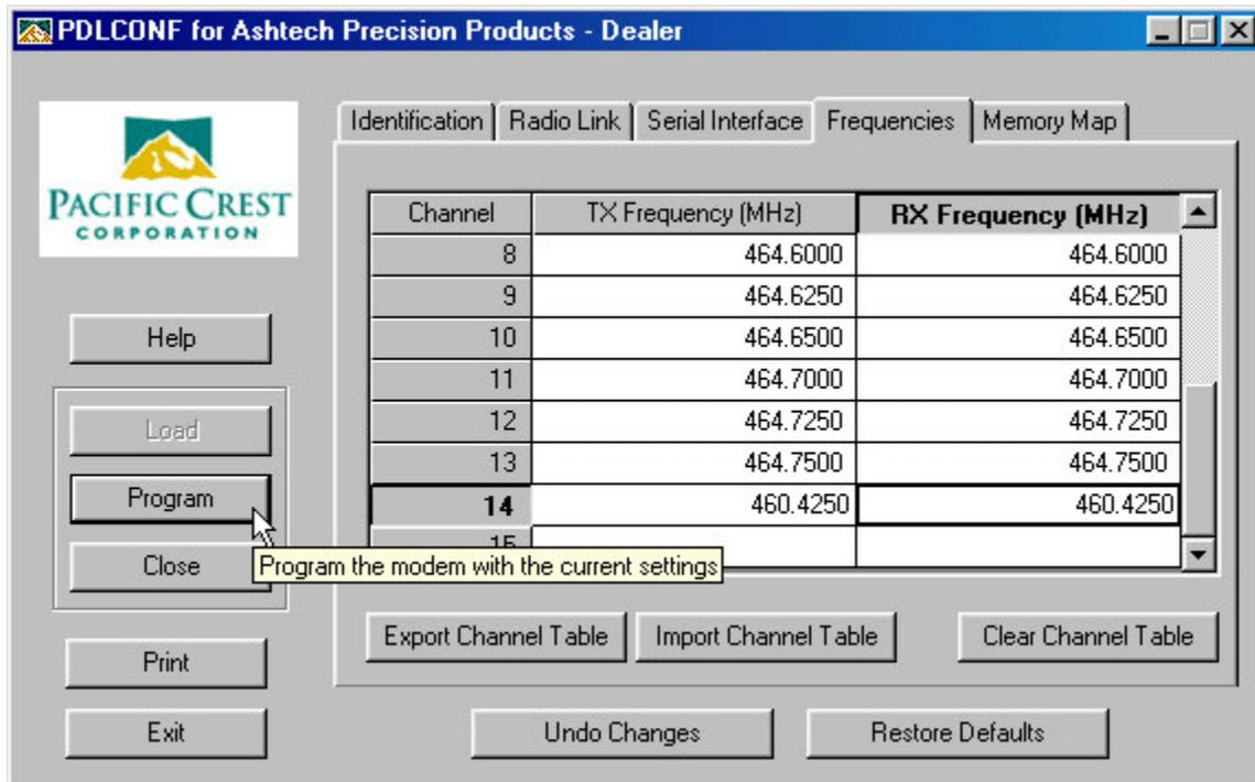
After manually entering the 460.4250 Mhz frequency to the TX and RX template, click on the "PROGRAM" button bar...
