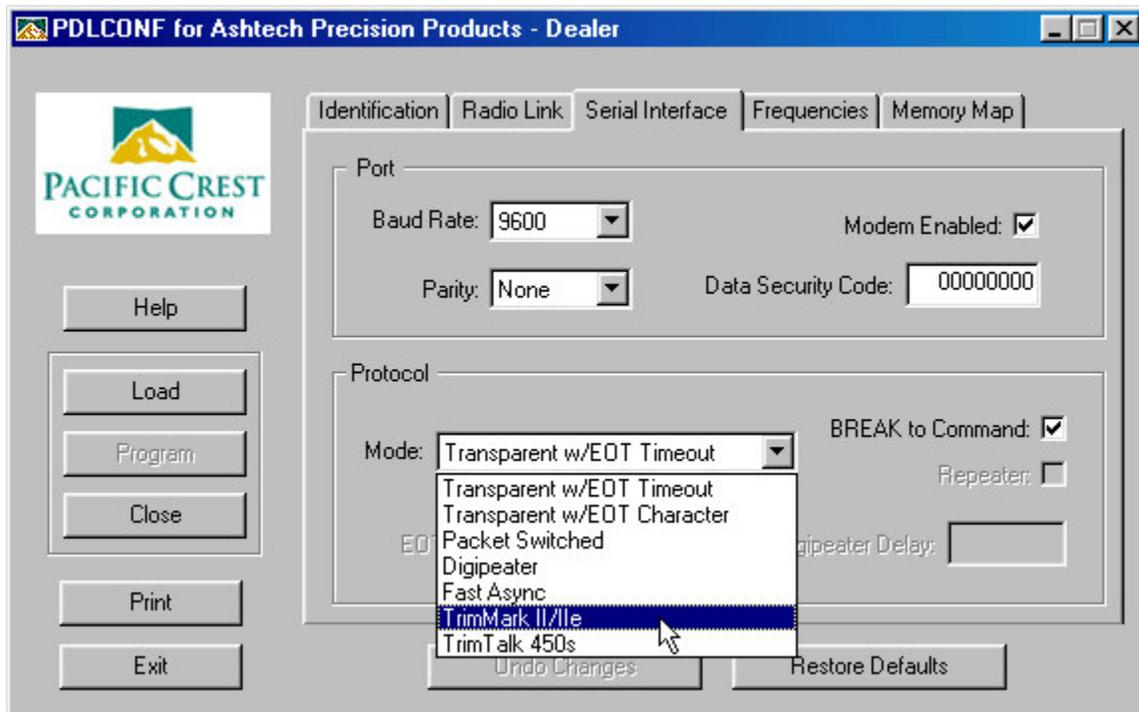
**Depending upon the type of Trimble radio being used at the Trimble RTK Base Station location select:**
