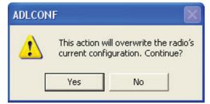
Click **Yes** to copy the default settings from the radio's permanent memory to the computer RAM for review and editing. The radio does not use any changes until you click **Program** in the main dialog or in the *Exit* dialog. When restoring factory defaults, the ADLCONF current channel table is retained.
