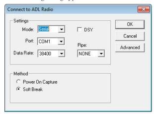
5. To connect to an ADL radio that is connected to the PC via a serial cable, select Serial in the Mode box. Then, select the COM port that the radio is connected to (from the *Port* list) and then select a baud rate (from the *Data Rate* list).
