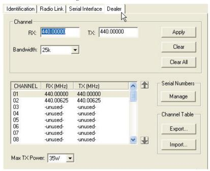
Use this tab to manage channel tables. Channel tables are lists of radio settings that comprise the following:
