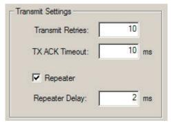
Enter the amount of time you want to elapse between receipt of a data packet and its retransmission. You may enter any value between 0 and 255.
