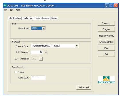
In this tab, you can configure the serial interface between the radio and external devices such as a computer running the ADLCONF software, a GNSS receiver, or monitoring equipment.
