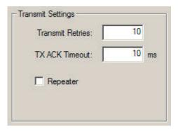
**Note** – Only Transparent EOT/EOC and Packet Switched protocols support transmit retries. So when you select any other protocol (on the Serial Interface screen described on page 21), the Transmit Settings section of the Radio Link screen displays only the Repeater check box.
