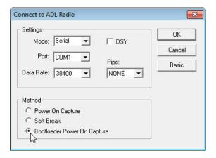
3. *Within 10 seconds*, turn on the radio. The bootloader firmware puts the radio into monitor mode that will accept commands.
