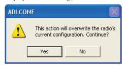
Click **Yes** to copy the default settings from the radio's permanent memory to the computer's memory for review and editing. No changes are made to the configuration the radio will use until you click either the **Program** button on the main screen or the **Program** button on the *Exit* dialog. When restoring factory defaults, the ADLCONF software keeps the current channel table.
