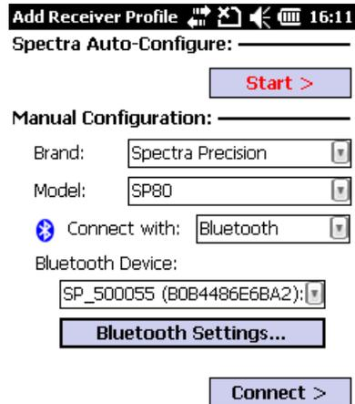
Make sure the new device is selected in the 'Bluetooth Device:' dropdown list.
