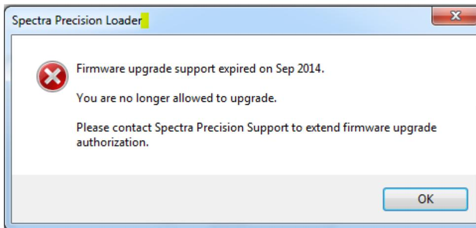
Note: Your Spectra Precision support will provide you an option code to extend the warranty period. Follow the “Upgrade Option” procedure to load this option, and start again the PM700 FW upgrade process.
