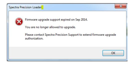
Note: Your Spectra Precision support will provide you an option code to extend the warranty period. Follow the "Upgrade Option" procedure to load this option code, and start again the ProMark 700 FW upgrade process.
