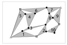
The observation plan shows that it will take 10 separate observation sessions to complete the survey based on the network design shown in *Fig. 4*.
