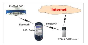
The CDMA connection is entirely controlled from the field terminal running FAST Survey.
