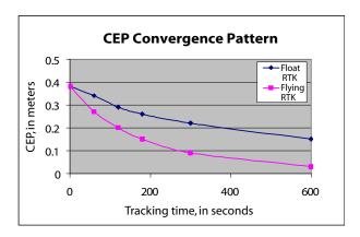
The CEP error (50% horizontal) is plotted vs. the time elapsed after BLADE was reset. The collected data include more than 150 reset operations for each of the different 22 baseline lengths used, which ranged from several meters up to ten kilometers.
