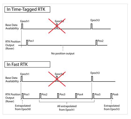
In the above Fast RTK mode example, the output rate has been set to twice the base data output rate.
