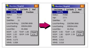
Other screens are available from within the **Monitor/Skyplot** function showing the details of the constellation, of the base position and of the RTK position solution:
