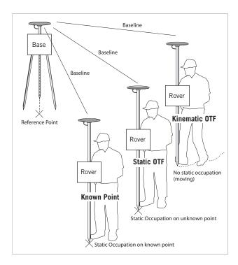
**Kinematic OTF.** For both post-processing and RTK real-time, this method does not make initialization faster but is the less constraining method in the field (although it does not release
