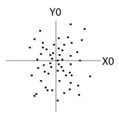
The origin of the (XO, YO) axis system is the true position of the reference point. Each dot represents a position solution delivered by the GNSS System for this point.
