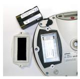
The battery used in the ProMark500 is a 7.4-V DC - 4400 mAh rechargeable battery. It is a standard model used in many camcorders.
