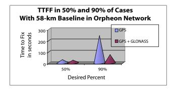
One can see that while 50% point of TTFF is almost equivalent for both cases, for 90% point there is a dramatic improvement thanks to using BLADE GPS+GLONASS solution. In other words, GLONASS being not so important in cases when GPS alone is good, is very important in worst cases when the power of GPS alone is not sufficient to get quickly fixed solutions.
