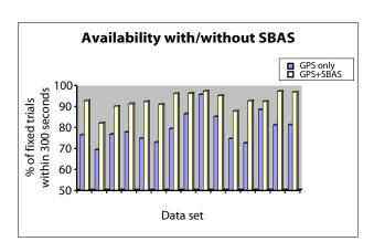
Using SBAS ranging in BLADE, the improvement is even more dramatic when processing baselines under medium/ heavy shading. SBAS satellites noticeably improve geometry and result in dramatic improvement in performance over the GPS-only case. The first two data sets correspond to medium sky shading, while the third one corresponds to heavy shading where a GPS-only solution is typically useless.
