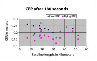
Again, L1 GPS-only data were used for evaluation. The plot shows that, even for long baselines, with only L1 GPS data, Flying RTK can deliver decimeter-level performance.
