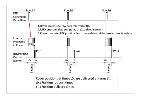
The time when position is requested is t0 and the time when the rover starts providing the position for time t0 is t1. Times t0 in the base and the rover are synchronous because they originate from the same clock which is the GPS System time. Here the latency (t1-t0) is caused by data processing times in both the base and the rover as well as the base-rover propagation time, the latter being negligible compared to the former. In this configuration, a typical latency time in
