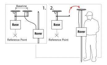
The Initializer Bar method can be used more especially when the survey takes place in the vicinity of the base (short baseline). It makes use of an initializer bar, also called "kinematic bar", mounted at the base. The bar is attached to the antenna base and, for a limited time, the rover antenna as well.
