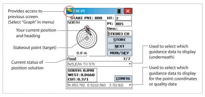
When the remaining distance is within the stakeout tolerance (this parameter can be changed in **Equip>Tolerances**), markers appear in the four corners of the target. You can now set a stake on this point.
