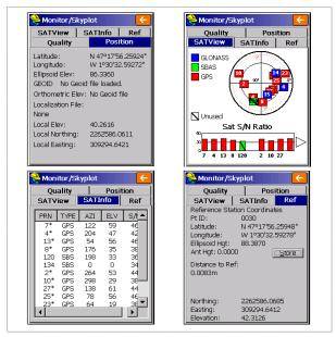
In NTRIP and Direct IP modes, a **Disconnect/Connect** button is available on the **Ref** tab to easily control the network connection. There is also a horizontal bar showing the GSM signal level until the modem is on-line. The bar disappears when the modem is online.
