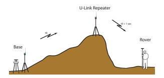
Assuming the U-Link repeater has been configured to operate with the U-Link transmitter you are using at the base and the U-Link receiver used in the rover<sup>1</sup>, do the following to operate the radio link:
