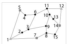
Fig. 7. Network Design for 15-Point Control Survey
