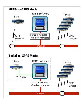
In Serial-to-GPRS mode, the base and the computer running RTDS are at the same location since a conventional RS232 serial line is used to connect one to the other.
