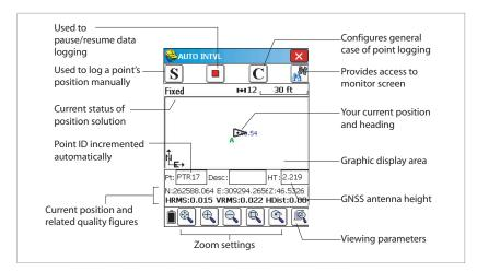
The **\$** button lets you instantly log the position of a point. The pause button allows you to pause data logging in continuous mode.
