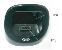
The top view of the docking station shows the slot **[19]** in which to insert the receiver from above the docking station. At the bottom of the slot is the 16-contact connector **[20]**. When resting on the docking station, the receiver is automatically powered from the AC adapter (if connected) and the charging status of its internal battery tested.
