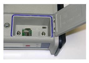
The battery used is a 7.4-V DC - 4400 mAh rechargeable battery. It is a standard model used in many camcorders.
