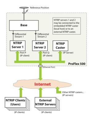
In its simplest configuration, the embedded NTRIP caster can be used to emulate the Direct IP mode (i.e. IP connection to a unique source of corrections), with the additional advantage that, contrary to conventional Direct IP, the embedded NTRIP caster can offer an effective protection of the source of corrections by restricting its use to the sole authorized users.
