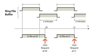
The Ring File Buffer continuously memorizes in turn two potentially deliverable sets of data, the duration of which corresponds to that requested for the G-file.
