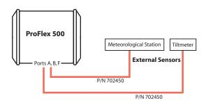
As the administrator, you can ask the receiver to initiate the communication with the external sensors in order to acquire data from these sensors. Initialization and trigger strings may in advance be assigned to the concerned serial ports for this purpose.
