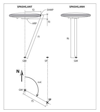
You will necessarily choose only one of these commands to define the ARP and discard the other. Whether the last command run is ANT or ANH, it will in any case supersede the settings made with the ANT or ANH command run previously.
