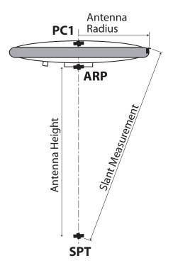
Through the \$PASHS,POS command, you can enter the exact position of the base and tell the firmware if it is tagged to PC1, ARP or SPT. The position you enter through this command is the one that will be transmitted to rovers, along with RTK differential messages.
