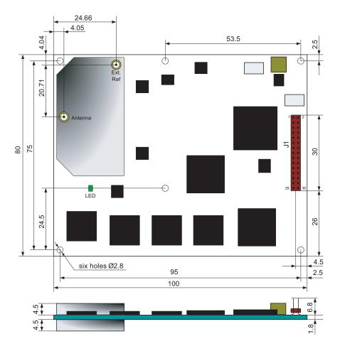
The board can be secured onto a chassis of your choice through 6 holes dia. 2.8 mm. The above diagram gives all the dimensions allowing you to perform this operation.
