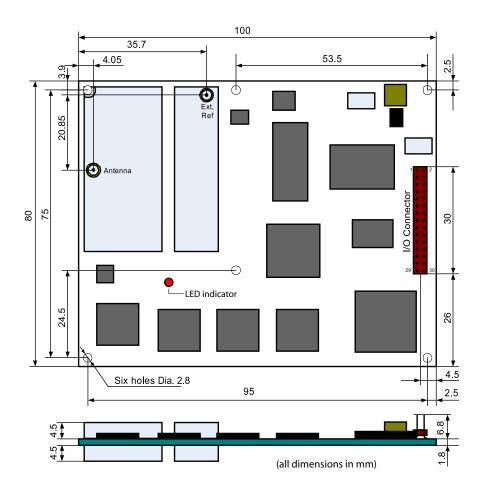
The board can be secured onto a chassis of your choice through 6 holes dia. 2.8 mm. The above diagram gives all the dimensions allowing you to perform this operation.
