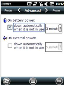
Another way of saving the battery is to allow the receiver to switch automatically to Suspend mode after a certain period of inactivity.
