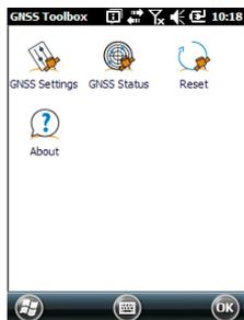
**GNSS Toolbox** is used to control and monitor important functions in your receiver. These are listed and detailed below.
