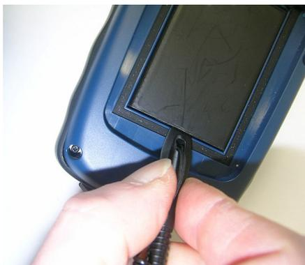
Likewise, extracting the SIM card or micro SD card from the battery compartment requires the use of a spiky-tipped tool to pull the card out of its slot.
