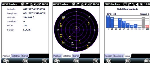
The default **Position** tab shows the latitude, longitude and altitude of the current position, as computed by the receiver, as well the number of satellites used and the current PDOP value.
